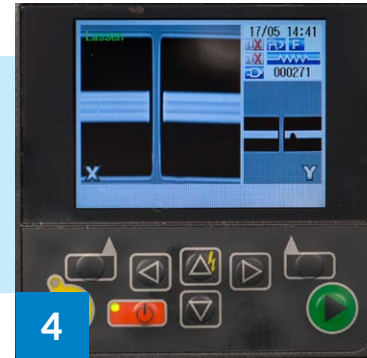
4 The display shows the quality of the fusion splice
